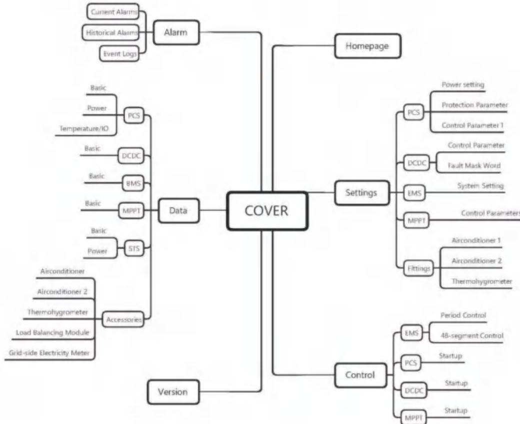
Figure 7-1 HMI Screen menu logical structure distribution diagram
