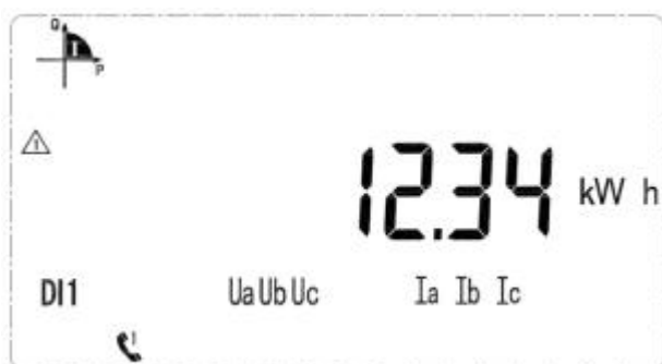
Current forward active energy 12.34kWh
