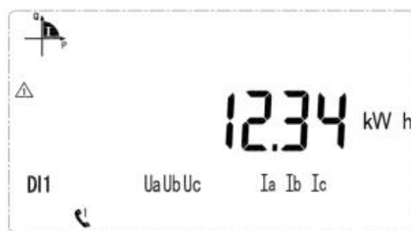
Current reversing active energy 12.34kWh
