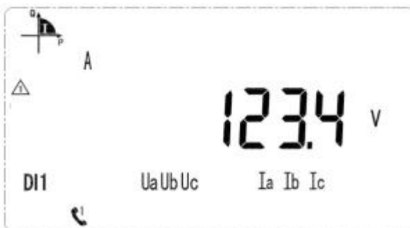
Voltage on A phase is 123.4V
