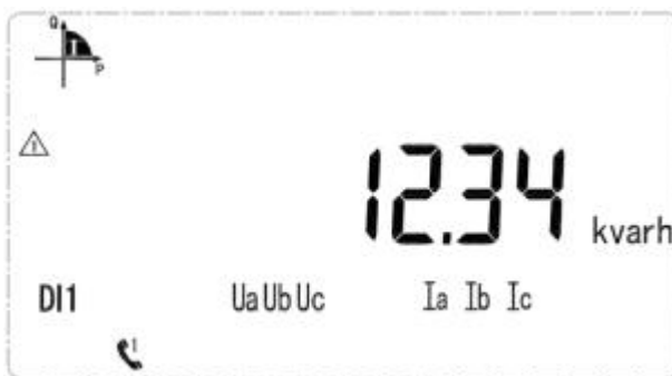
Current forward reactive energy 12.34kWh
